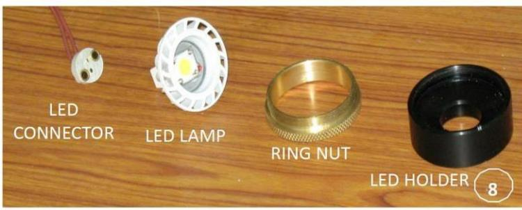
Fig 8 Remove the LED Connector & Ring Nut
